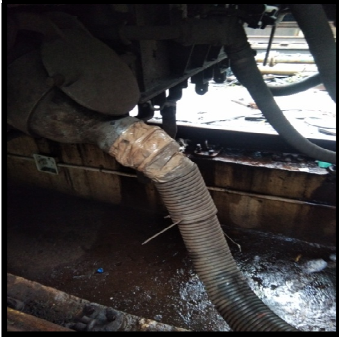
750 volts damaged cable pipe in the LHB formation came to BBQ yard
