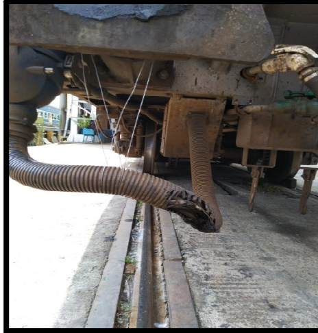
750 volts damaged cable pipe in the LHB formation came to BBQ yard
